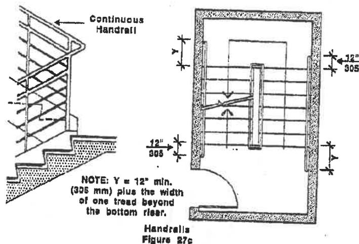
27.4.2 Height: Top of handrail gripping surface shall be mounted between 34 inches (34" = 864mm) and 38 inches (38" = 965mm) above stair nosings.
